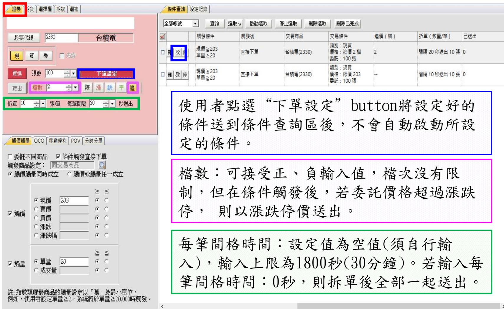
The screenshot displays the '證券' (Securities) section of the trading platform. On the left, the '股票代碼' (Stock Code) is set to '2330' (台積電). The '下單設定' (Order Settings) section includes '買進' (Buy) and '賣出' (Sell) buttons, with '張數' (Quantity) set to 100 and '拆單' (Split Order) set to 10. The '觸發條件' (Trigger Conditions) section is set to '觸發觸量同時成立' (Trigger on volume simultaneously) with '觸價' (Price) set to '現價' (Current Price) and '觸量' (Volume) set to '單量' (Quantity) with a value of 20.
